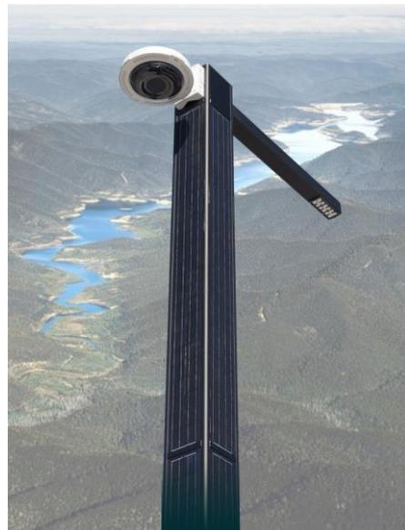
In addition to the fixed tower-based solution being provided to Melbourne Water, EYEFI will be deploying the first of the vantage point cameras this coming fire season; offering entirely new vision and spatial targeting of fire ignition events located in remote areas of the water catchment. The innovative solution incorporates the solar panel into the pole design and houses all EYEFI communications equipment and batteries, to provide 24/7 monitoring of the surroundings.
